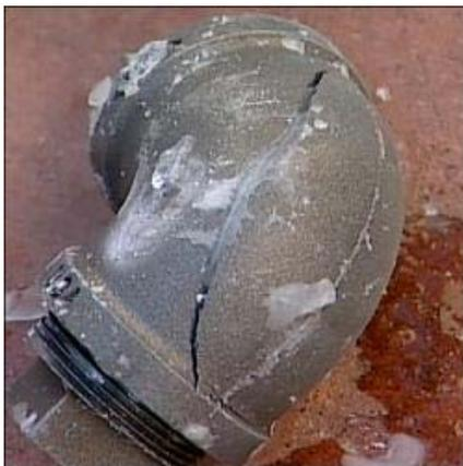
Fittings like this iron elbow are designed to handle water pressure well in excess of 250 psi. However, they are no match for the tremendous forces generated as freezing water expands into ice. The water damage from a split fitting can add up to tens of thousands of dollars.
