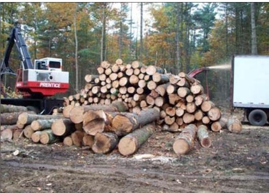
Today's logger utilizes nearly every part of the tree in a highly efficient and environmentally friendly manner. Wood that isn't suitable for saw logs or fire wood is chipped and blown into trailers (shown above) and can be used for making paper, wood pellets, wood gas or burned directly as biomass.
