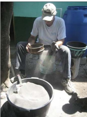
Norm sifts sand for hours to obtain the correct particle size. Sand filtration is documented as far back as 2000 BC by the ancient Greeks.
