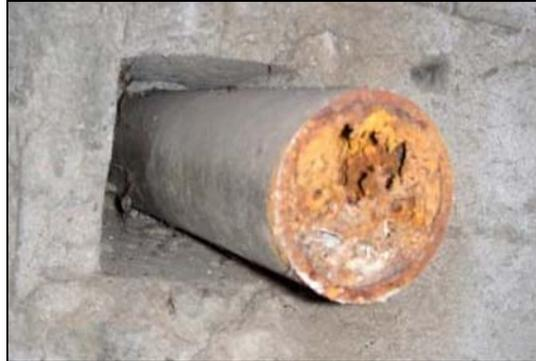
Water can barely get through this heavily oxidized (rusty) private galvanized iron pipe service line.
