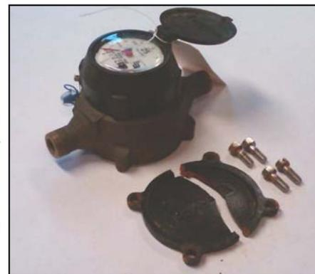
The base plate on this 5/8" meter is rated for 150 psig but was no match for the forces caused by freezing. Replacing a frozen meter like this could set a customer back over \$150.
