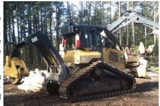
The tracks on this grapple skidder distribute weight much more effectively than standard rubber tired models, thereby eliminating ruts and reducing soil erosion.
