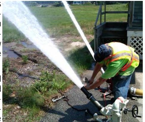
District Trustee and retired Kennebunkport Fire Administrator Jim Burrows calculates the available flow rate after the new 16" water main was installed at Goose Rocks Beach (Kennebunkport) in 2010. The new 16" main has more than doubled the available fire flow by replacing an obsolete and undersized 1927 vintage 10" main.
