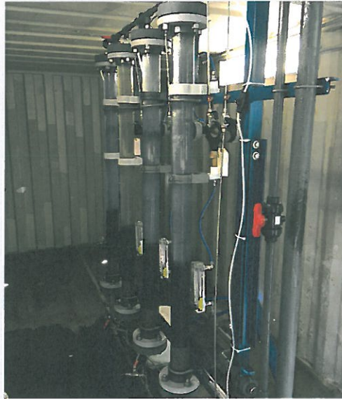
One of our pilot study setups comparing the performance of four types of GAC
