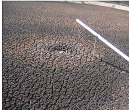
Step 2. Surface water evaporates during the hot summer months leaving a two foot thick pudding-like "sludge" behind.
