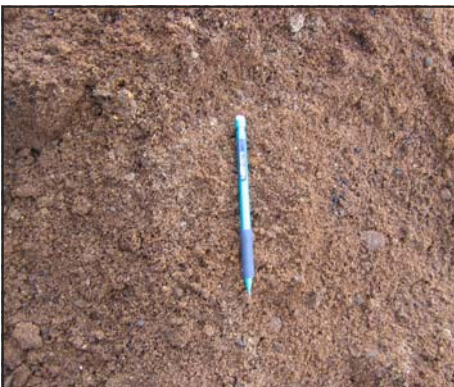
Step 4. The freeze-drying process transforms the "sludge" into hydrosolids that look and feel similar to coffee grinds.
