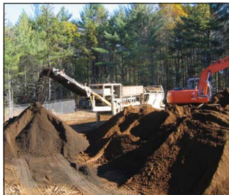
Step 5. A rotary drum screen is used to blend hydrosolids, compost and loam to manufacture a high quality topsoil.
