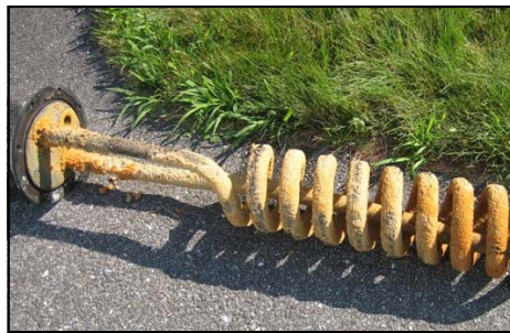
The calcium deposits on this hot water heating element act like insulation, driving up your heating costs. Clean or replace the element.
